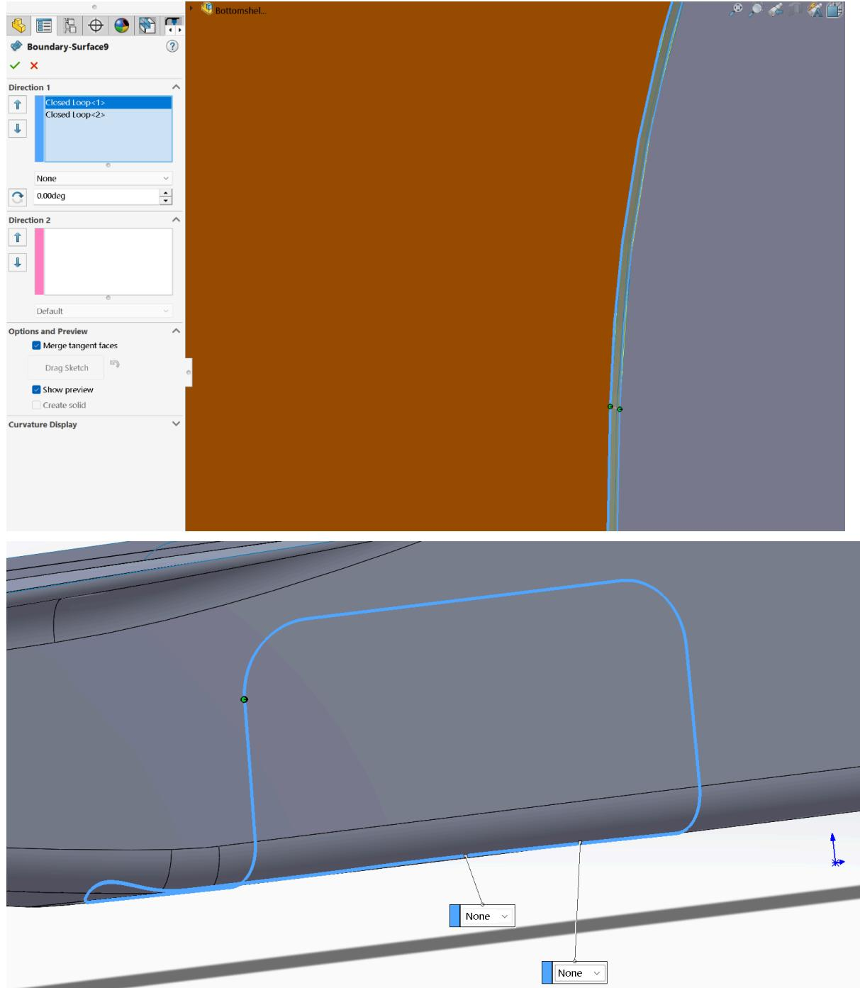
Repeat this process for all four fairings and the battery access panel. Make sure to knit each indent to the rest of the car as you progress through.
