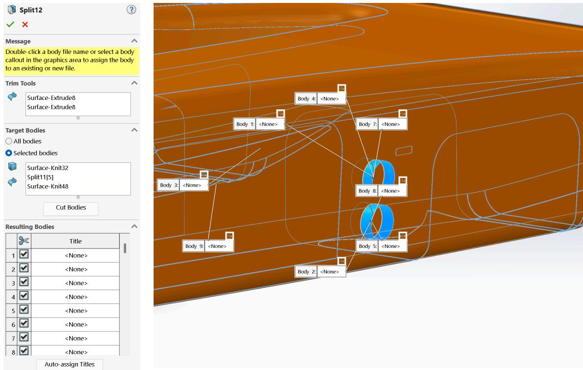
Then as per usual, create the boundary surface and knit everything together. Repeat this process for the exhaust duct on the inside of the hull.
