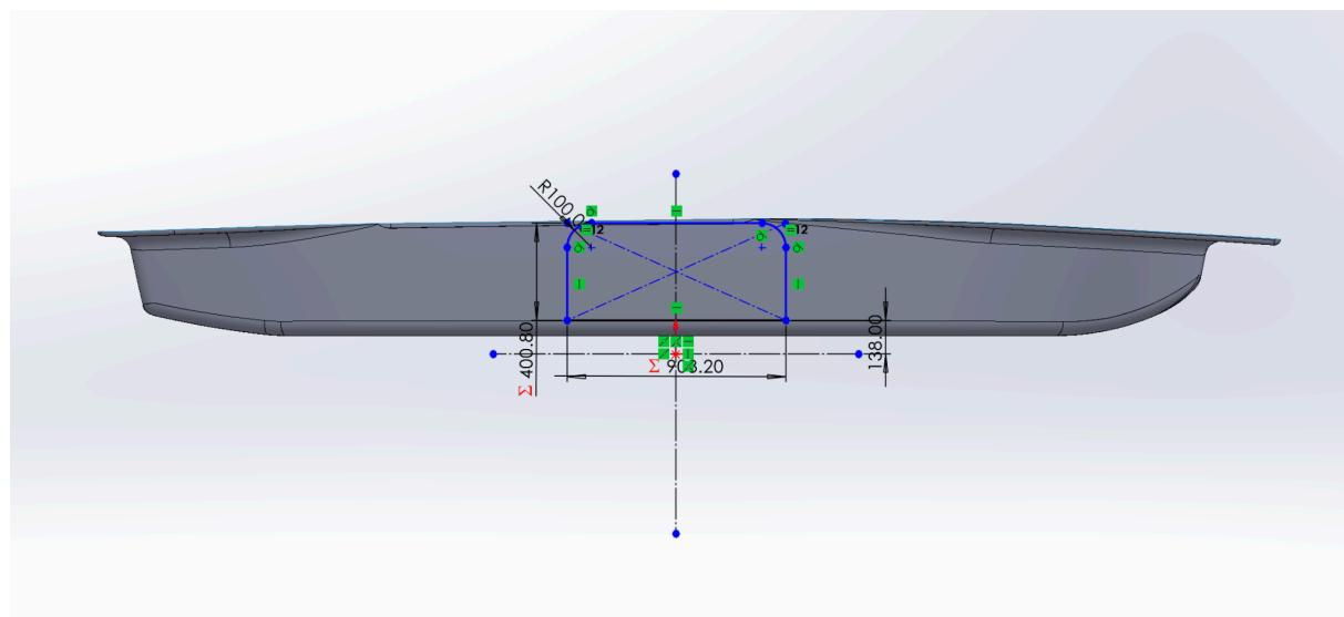
Once you do this, you want to split the aeroshell and the 1.5mm offset. You are going to split it twice. The first split, you want to select the sections referred in the image below. These would be the inside of the car except the area where the fairings split, and then the outside where the fairing is.
