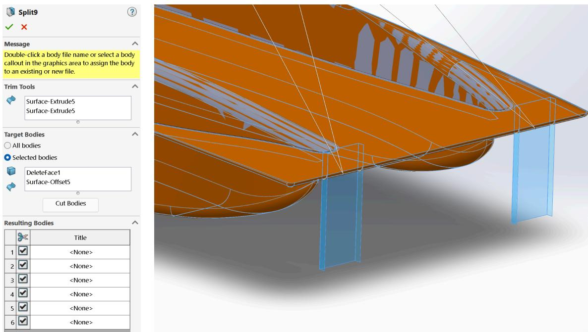
Select the delete bodies features and delete the u-shaped surface extrudes, along with the original aeroshell surface that has been split.
