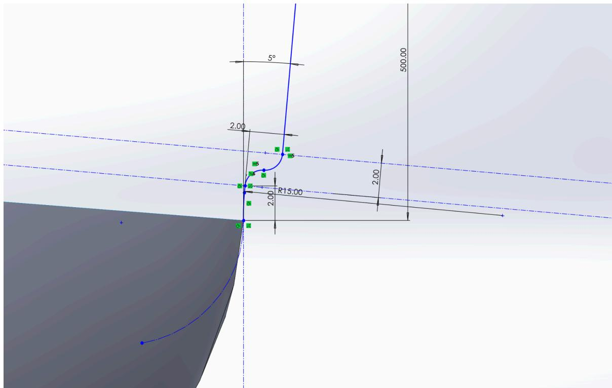
Then create a 3D sketch that runs along the path of the back of the car. You can use the convert entities feature to make this easier.
