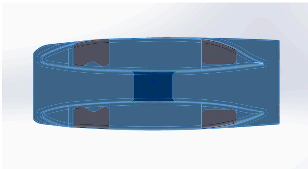
Next, you wanna make all of your boundary surfaces for each fairing. It “should” be a simple process. First, try selecting each loop on its own to see if Solidworks is nice and will create a closed loop for you automatically. In my case it did not, so I created a 3D sketch that outlined the two loops that I wanted to surface between.
