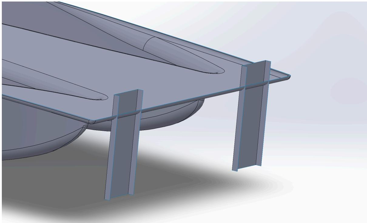
Once that is done, find the split tool feature. Use the two extruded U-shapes as the trim tool and select both the original aeroshell surface, as well as the 1mm offset as the bodies to trim. Select cut-bodies. Select all cut pieces.
