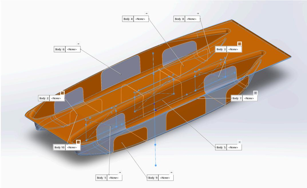
Next you want to split it again, but this time only selecting the outside of the fairing and the inside that is not going to be fairing. This is because the split will cut through the inside of the hull and the outside of the hull. In the end you only want it to split the outside. So by doing this, you can knit together the rest of the pieces after. The photo below shows this second split selection, and the photo after that is the same split but another angle.
