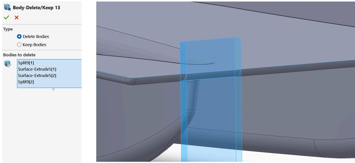
You now want to create a boundary surface between the 1mm offset face and the original aeroshell body. This can be tricky. It is best to create a 3D sketch in this scenario to draw out the lines in order for Solidworks to not get confused.
