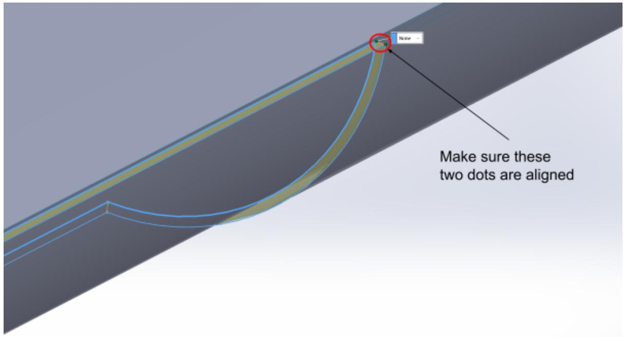
Finally knit everything together (the original aeroshell, the offset surface and the boundary surface)
