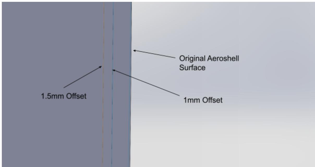
If you are having issues with failing faces, you can use the delete face feature to help fix that. When you encounter failing faces, it is usually because there are small faces that intersect with the car when offsetting. Due to how small these faces are, we can delete these faces and patch them with minimal geometry change. Refer to the bottomshell plug issues tab in this document for further details.
