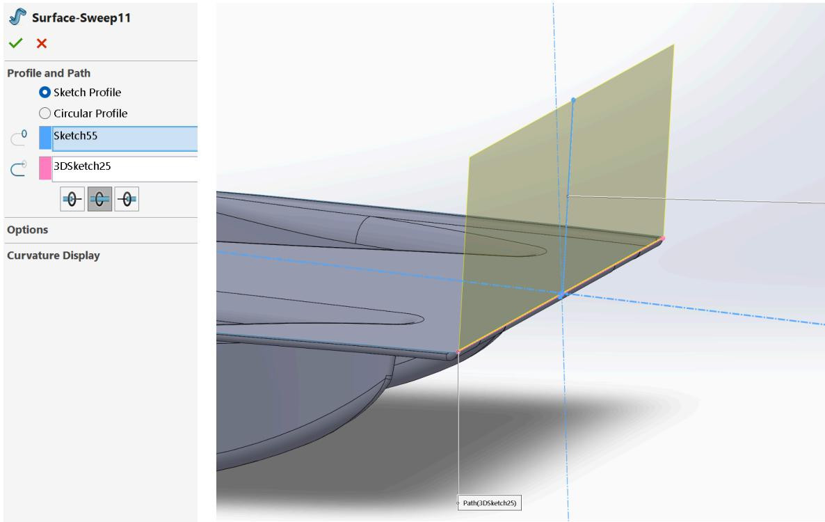
Then knit the surface to the rest of the car, and that's one side done.
