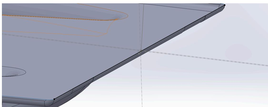
Then use the surface sweep feature. Select the profile on the right plane as the profile and then the 3D sketch as the path. Make the surface run both ways.
