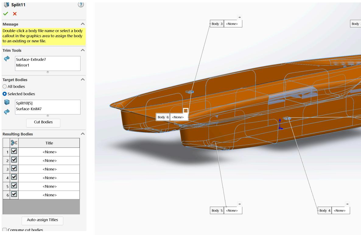
Finally knit everything together (the original aeroshell, the offset surface and the boundary surface)
