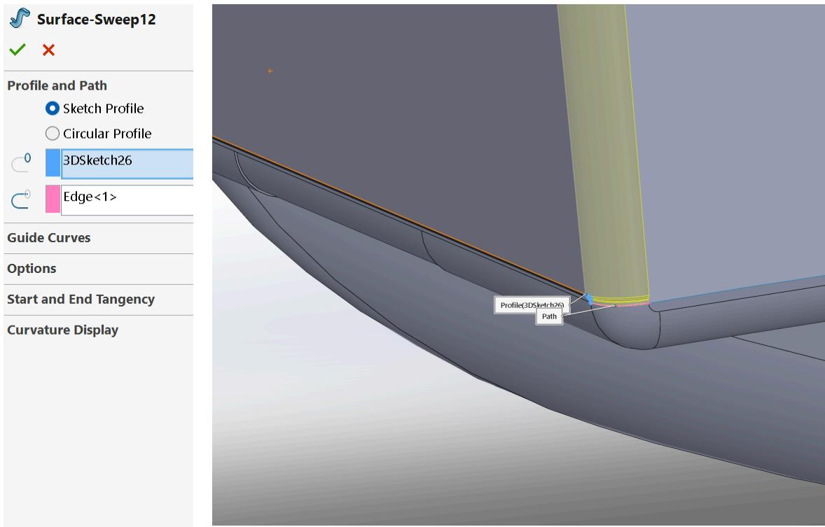
For the sides of the car, you have to add that profile at the end, middle and front of the car. Then you have a 3D sketch that is the guideline between all three of those. Then surface loft it and select the three extension profiles with the 3D sketch as your guideline. For the middle sketch I used the front plane for sketch reference. For the front I created a reference plane at that point.
