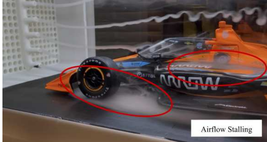
Figure 27: Front From Rear, 25% Fan Speed(200RPM)
