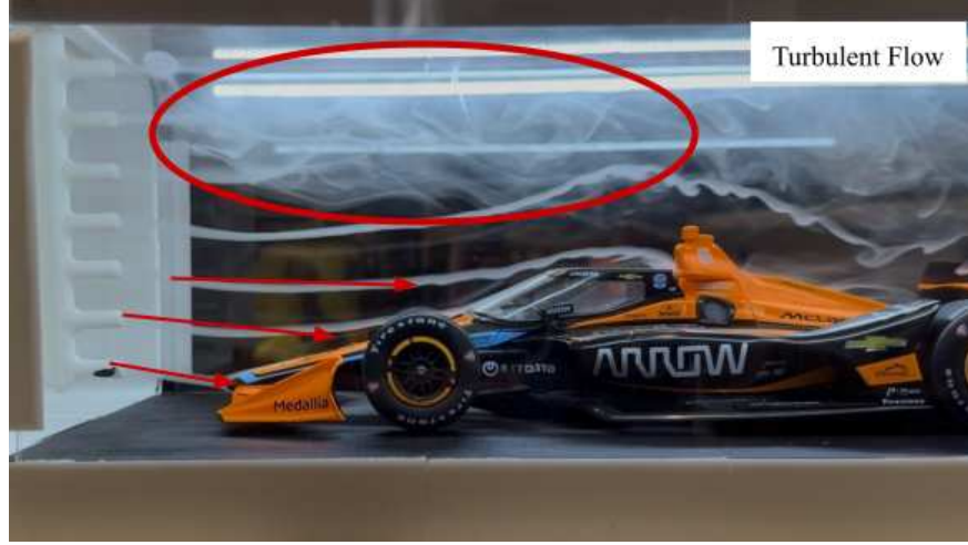
Figure 26: Sideview, 25% Fan Speed(200RPM)
