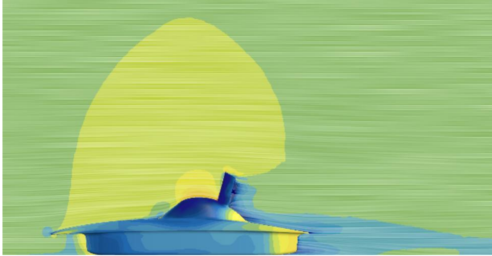
Figure 24: Canopy side velocity vector flow field
