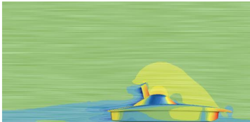
Figure 21: Right side velocity vector flow field
